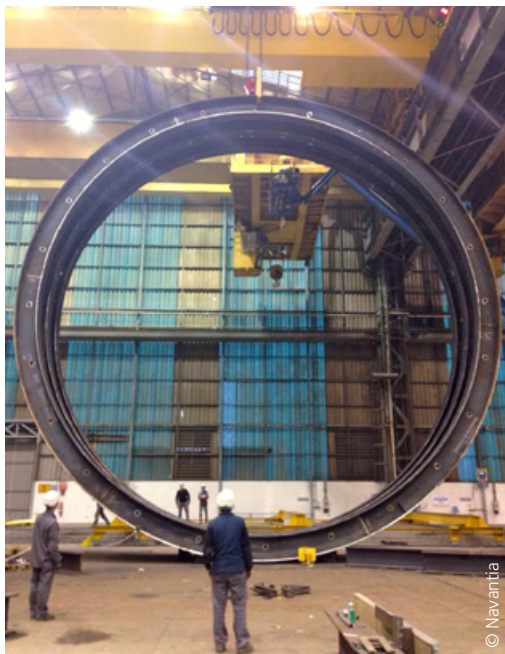
A series of steel rings form two watertight compartments which provide flotation and stability.
