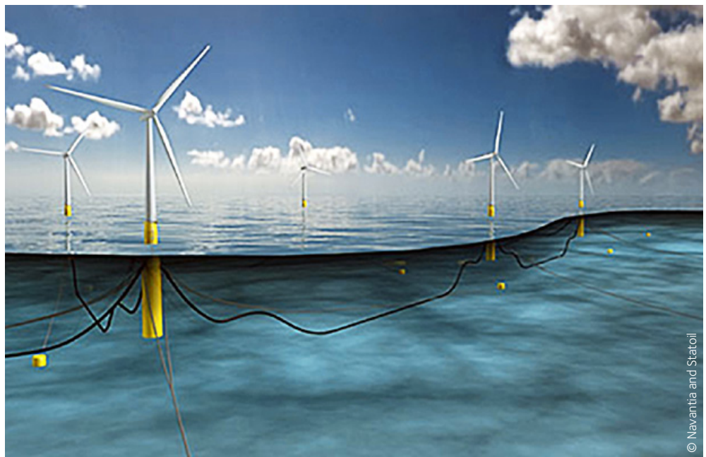
Each floating turbine is anchored by a series of mooring lines.
