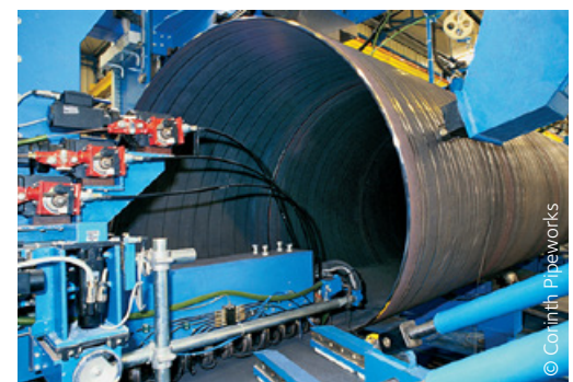
Pipes undergoing helical submerged arc welding (HSAW) at CPW.
